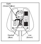
This appliance is equipped with a plug fitted with a 13 amp fuse. Should the fuse fail, then it must be replaced with an ASTA approved fuse (conforming to BS1362) of the same rating. If you need to replace the plug or if the plug is of the incorrect type for your socket, remove it and replace it with an appropriate type. Dispose of the old plug safely.
