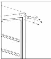
7. Screw the alternative left top hinge (included in the fittings) to the top left corner of the wine cooler and tighten securely.
