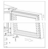
5. Gently remove the upper door and set it on a non scratching surface with the outside up to avoid the risk of damage.
