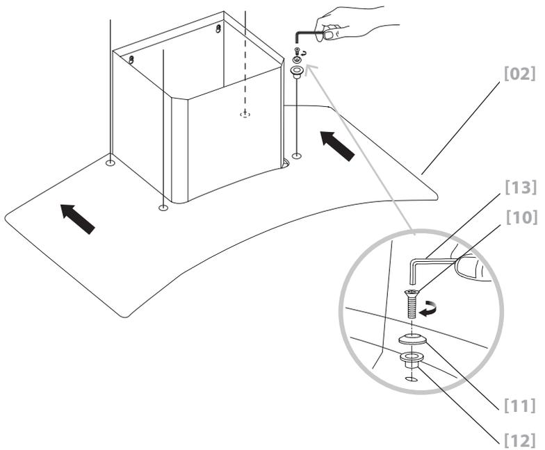
Tighten all screws (do not over tighten).
